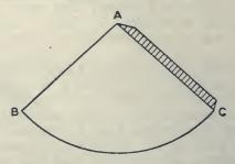
This sector is rolled up so that AC lies along AB, while the adjoining flap is gummed underneath. They must next make the corresponding cylinder. For this they must
